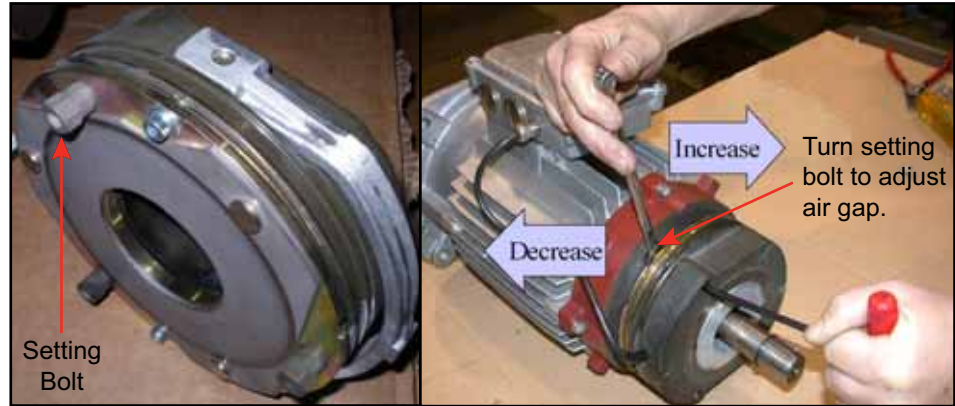
Figure 6-2: Adjusting the Setting Bolt
